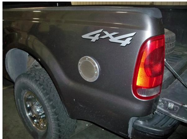
(Fig. 16) Fuel Door located in outside fender.
