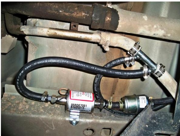
(Fig. 15) Vent Fill Neck Adapter installed.
