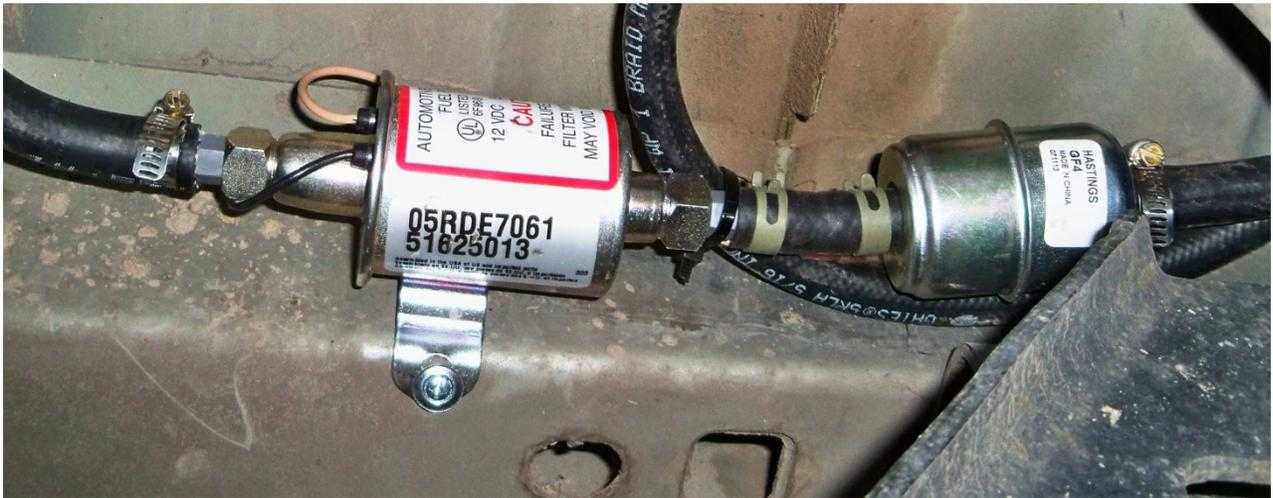
(Fig. 14) Fuel pump and inline filter installed.
