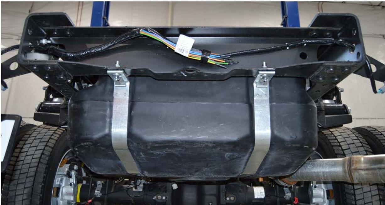
(Fig. 3) Rear of vehicle, showing how tank straps are attached to the frame.
