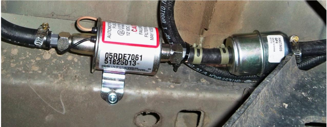
(Fig. 8) Fuel pump and inline filter installed.
