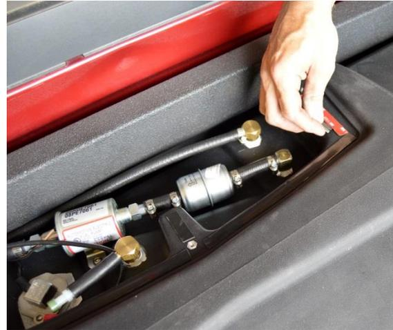
(Fig. 17) Showing completed plumbing and wiring on tank body. Tape backing is being removed in preparation for installation of the cover.
