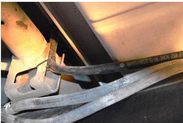
(Fig. 9) One of the vent hoses routed up and attached to the vehicle's body with quick tie.
