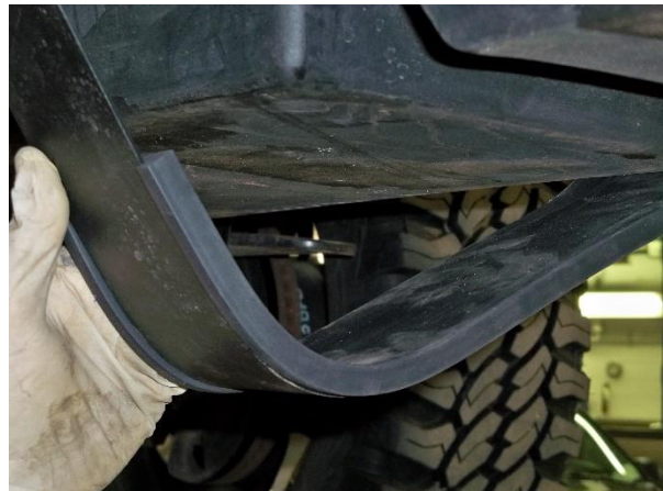
(Fig.14) Extruded bushings installed on straps
