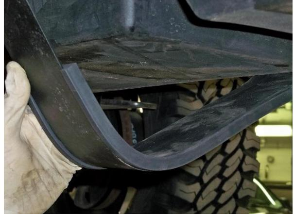
(Fig.12) Extruded bushings installed on straps.
