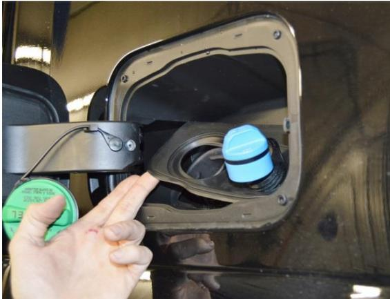
(Fig. 1) Loosen and remove rubber seal.
