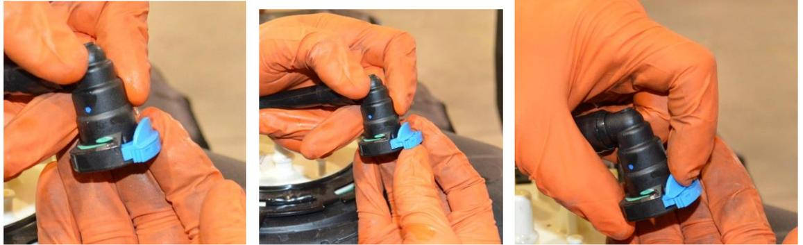
(Fig. 7): **Method for Disconnecting Fuel Line Couplings:** The majority of the couplings involved in this installation are of the quick connect type shown in left photo above. To disconnect, a) Slide the tab that has teeth on its edge outwards as shown in the center photo. b) Next, press the rounded button, as shown in the right photo, and pull the coupling apart. The coupling shown in Fig. 5 functions differently, see Step no. 9 for it.
