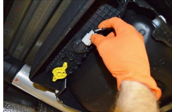
(Fig. 4) Disconnect electrical connection on the bottom of the water separator.
