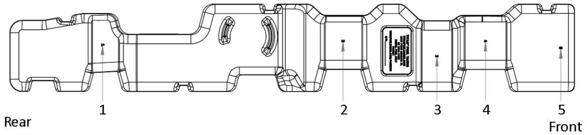
26 The top brackets and hangers must be installed before the tank body is lifted into the vehicle. These include A1, C, D, G1, and G2. Please view the images below as they depict placement and direction. As stated above, straps and supports will vary depending on application.
