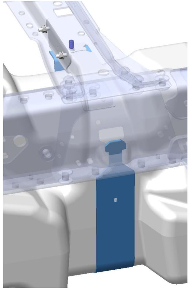
Fully installed A2 Rear Strap on all configurations. 1qty 3/8-16 x 1.5" Cap Screw, 1qty U Nut, 3/8"-16 0.75" center and 1qty 3/8"-16 Washer will be used. (02 0000 0456, 02 0000 0428 & 99 0000 0682)
