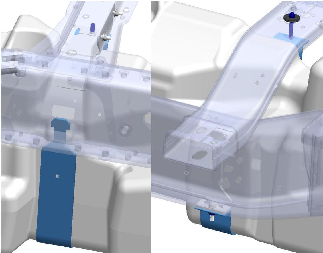
Fully installed B Front Support on 108 CA. 1qty 3/8-16 x 1.5" Cap Screw, 1qty U Nut, 3/8"-16 1.125" center and 1qty 3/8"-16 Washer will be used to connect to C bracket. (02 0000 0456, 02 0000 0430 & 99 0000 0682)
