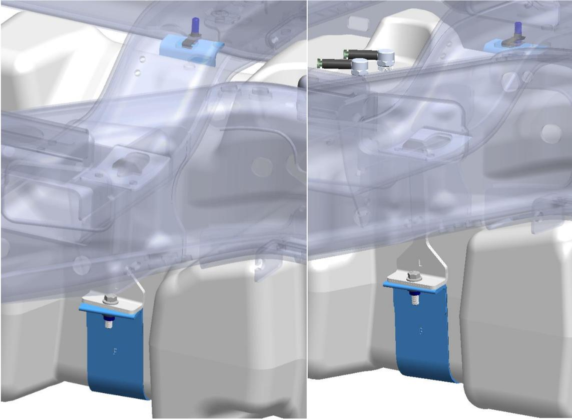
Fully installed F Strap on 60 CA. 1qty 3/8-16 x 1.5" Cap Screw, 1qty U Nut, 3/8"-16 1.125" center and 1qty 3/8"-16 Washer will be used to connect to the frame. (02 0000 0456, 02 0000 0430 & 99 0000 0682)
