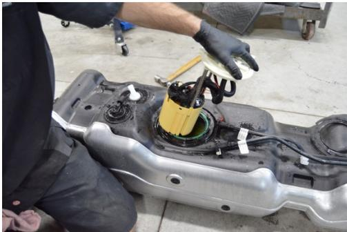
(Fig. 6) Remove the sending unit.
