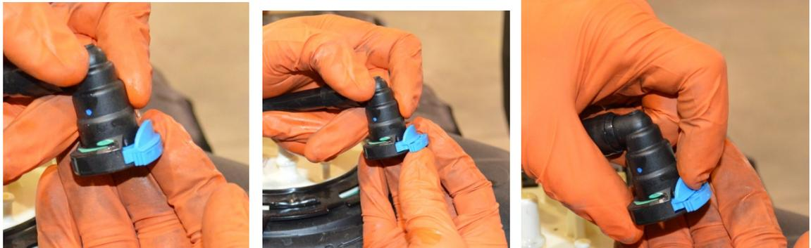
(Fig. 3): **Method for Disconnecting Fuel Line Couplings:** The couplings involved in this installation are of the quick connect type shown in left photo above. To disconnect, a) Slide the tab that has teeth on its edge outwards as shown in the center photo. b) Next, press the rounded button, as shown in the right photo, and pull the coupling apart.
