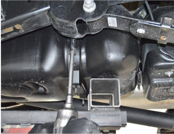
(Fig. 4) Remove OEM straps.
