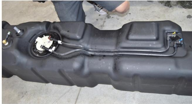
(Fig. 9) Fuel lines installed on the new TITAN tank.
