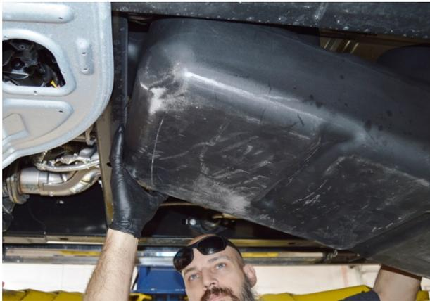
(Fig. 10) Angle tank slightly as it is lifted in so that front protrusion on tank slides over cross-member.
