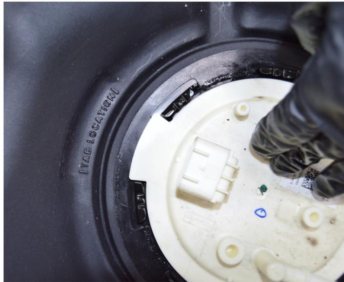
(Fig. 7) Line the tab on the sending unit up with the tab location marks on the TITAN tank.
