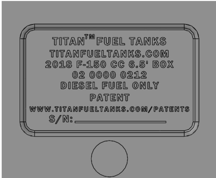
**Note:** The tank body has the above identification on its bottom. Please check to be sure the tank is properly identified as the one to fit your vehicle.
