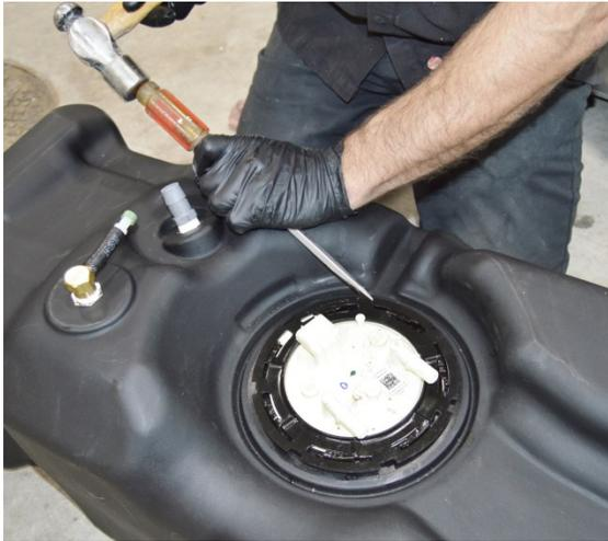
(Fig. 8) Use the OEM hold-down ring and tighten it by turning it clockwise as far as it will go.
