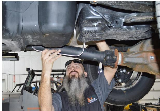
(Fig. 11) To install the new straps, turn and hook on inboard side of the tank, then rotate. Then tighten bolts on the outboard side.
