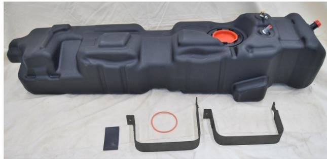
***Extended Capacity Replacement Tank for FORD F-150 Pickup Trucks with Power Stroke Diesel Engines, Crew Cabs, and 6.5 ft. Beds***
