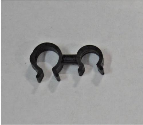
(Fig. 7) Remove the hose clip from the lines leading to the sending unit. Clip shown above.
