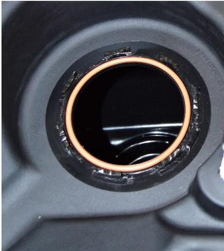
(Fig. 3) O-Ring gasket shown installed correctly.
