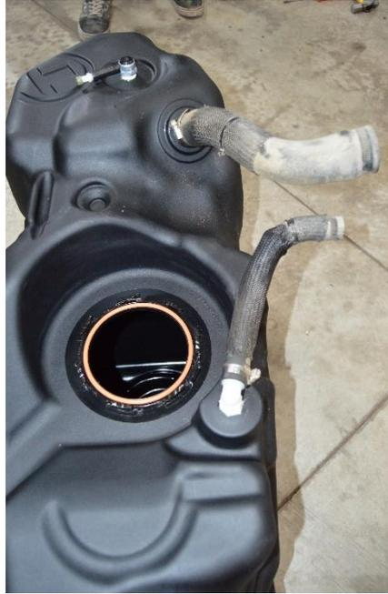
(Fig. 6) Install fill and vent hoses from original equipment tank on TITAN tank as shown. Make sure that they are lined up with orientation marks on the tank.
