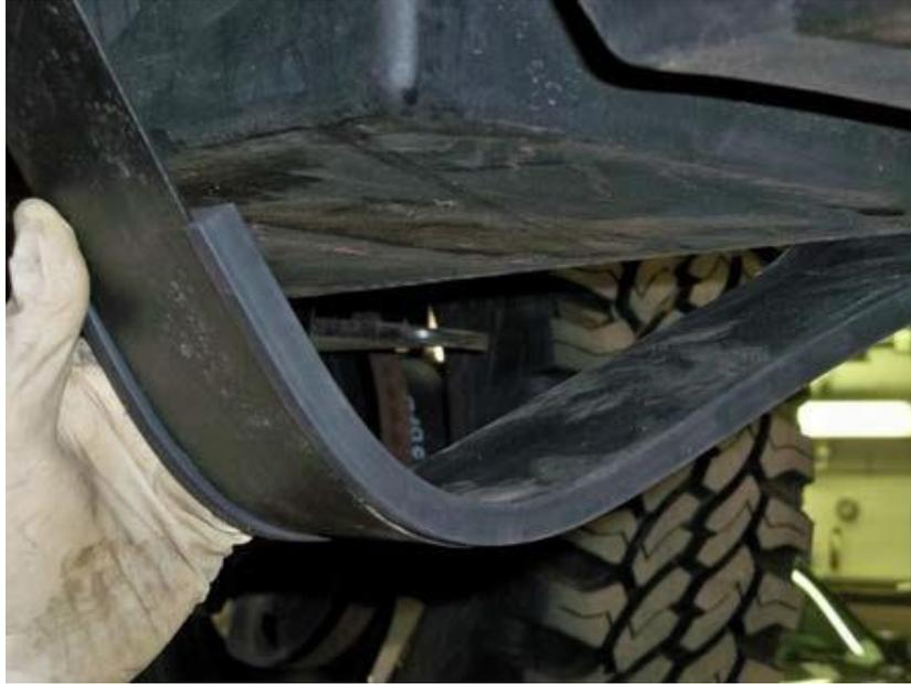
**(Fig. 6) Install Rubber Strap Bushings in tank mounting strap. Center the bushings in the bottom of the straps.**
