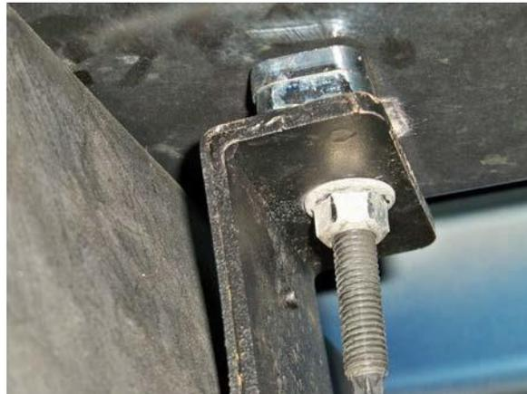
(Fig. 13) Thread two shims onto each strap bolt. (Fig. 14) Tighten the bolt and bracket against the shims. If the strap does not hold the tank tightly enough, remove one shim at a time until it is tight.
