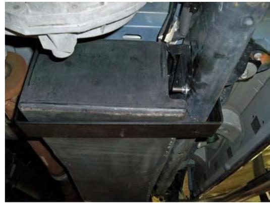
**(Fig. 12)** Photo shows the "S" Bracket Support installed at the front of the tank.
