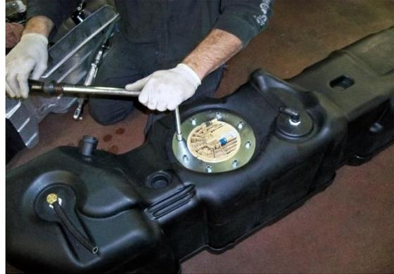
(Fig. 3) Place the sending unit into the TITAN tank, install the top flange, and tighten the nylon lock nuts to 20 ft. lbs using a "star" pattern using a torque wrench.
