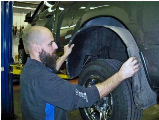
(Fig. 1) Some vehicles may require the removal of the fender liner and perhaps the left rear wheel so as to facilitate access to the tank fill and vent hoses.
