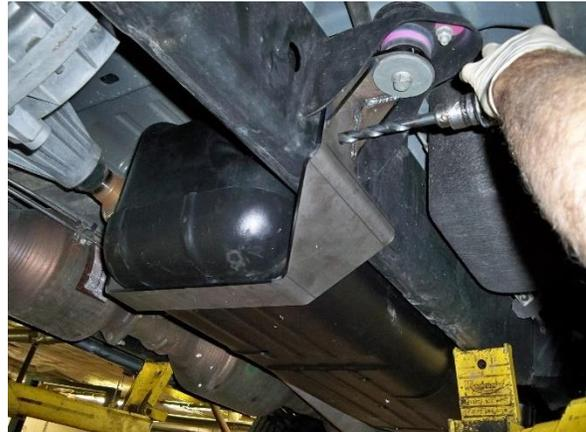
(Fig. 5) On 7030210 (Crew Cab, Short Bed) tanks only, bolt the Front Support to the nearest cab mount (as shown above), then use a ½” drill bit to drill through the support hole and through the vehicle’s frame. Bolt the support to the frame using the bolt and hardware provided.
