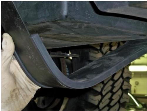
(Fig. 5) Install rubber bushings (pn 99 0000 0103) on both straps and the front Support with the channel side toward the strap.
