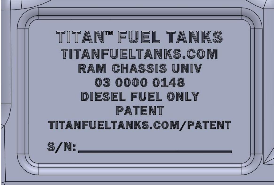
**Note:** The tank body has the above identification on its bottom. Please check to be sure that the tank is properly identified as the one to fit your vehicle. Notice the serial number space. You will need the serial number to register for warranty coverage.
