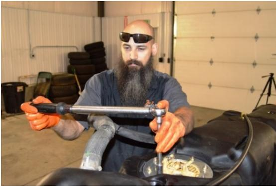
(Fig. 3) After placing the sending unit into the TITAN tank, install the top flange, and tighten the nylon lock nuts to 20 lb. ft. using a "start" pattern using a torque wrench.
