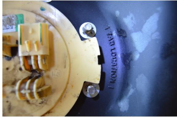
(Fig.2 ) Be sure the tab on the sending unit lines up with the "TAB LOCATION" marks on the body of the TITAN tank as shown above.
