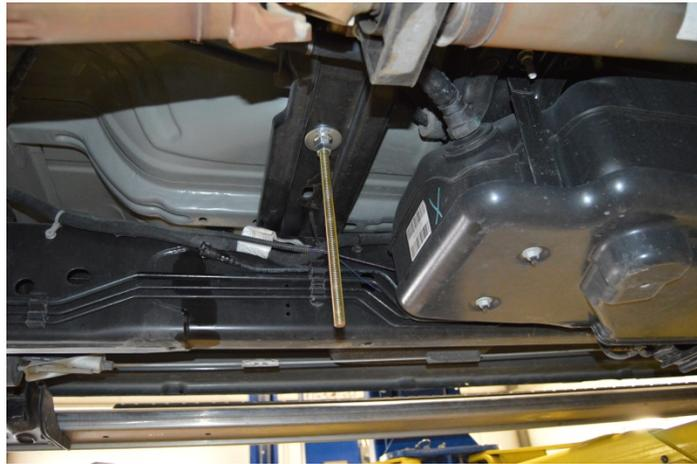
(Fig. 6) Install the “Threaded Rod” from the “Front Support Assembly” in the cross member just behind the DEF tank.
