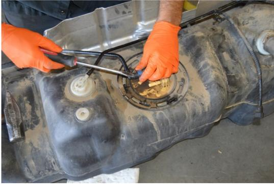
(Fig.1 ) Loosen the hold-down ring on the OEM tank by turning counter-clockwise.
