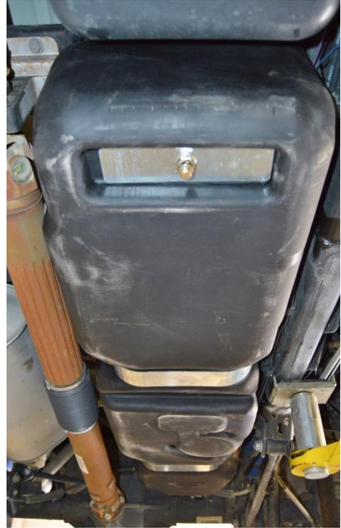
(Fig. 8) Tighten the "Front Support Assembly" to specifications. (Fig. 9) "Front Support Assembly" properly installed.
