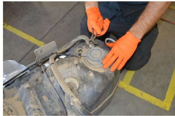
(Fig. 4) Using a pair of dikes, cut off the clamp holding the factory vent line. Remove the line, and the fill hose and install them both on the new TITAN tank.
