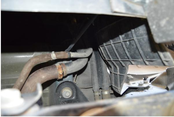
(Fig. 1) Loosen and disconnect fill hose and vent line from vehicle's fill spout.
