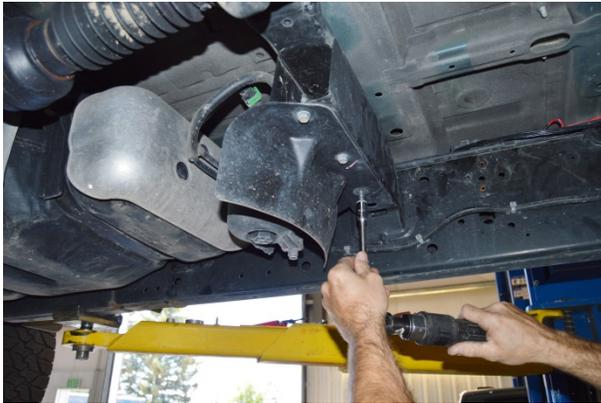
(Fig. 3) Remove shield from front of filter/water separator.
