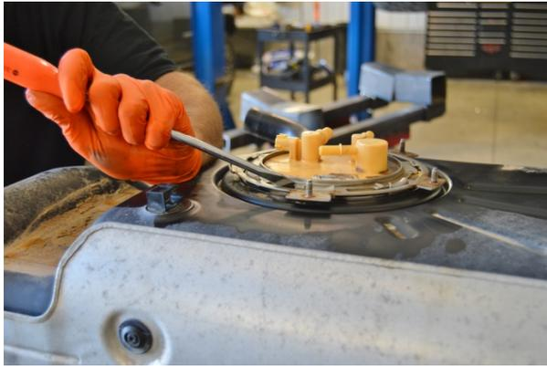
(Fig. 5) Loosen sending unit hold-down ring by turning it counter-clockwise.
