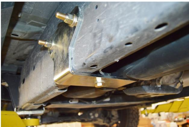
(Fig. 15) Front Support Bracket Installed.
