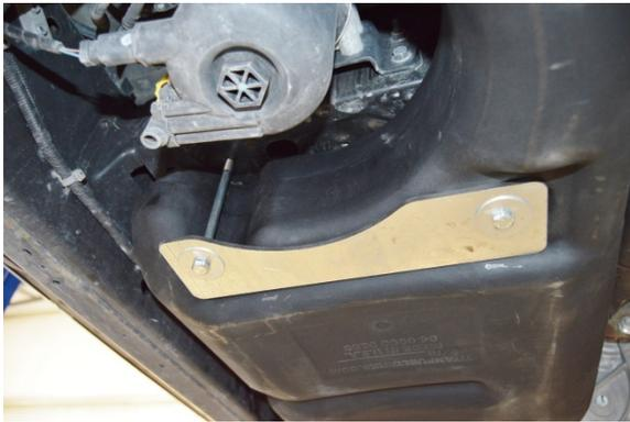
(Fig. 17) Center Point Mounting System installed.
