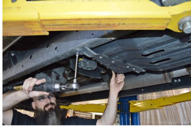
(Fig. 2) Remove factory shield.
