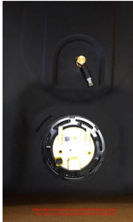
(Fig. 6) Orientation of Sending Unit in TITAN tank with Gen6 Torque Ring™: Be sure the electrical plug is pointing away from the tank vent and toward the front of the vehicle as shown.
