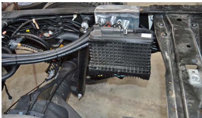
(Fig. 8) Water separator mounted on TITAN Mounting Bracket.
