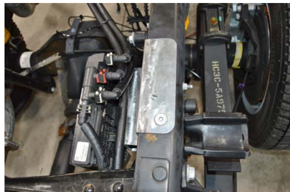
(Fig. 9) Top view of TITAN water separator relocation mounting bracket installed on vehicle frame.
