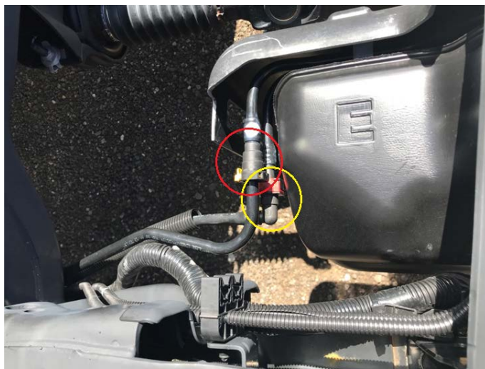
(Fig. 2) Fuel line connections at front of tank.
