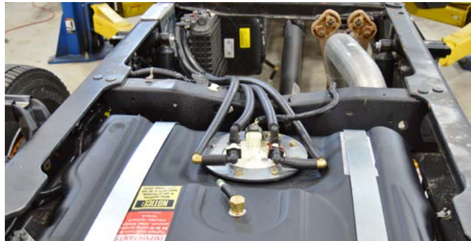
(Fig. 16) Hose routing from sending unit to water Separator (older Gen V mounting system shown).
