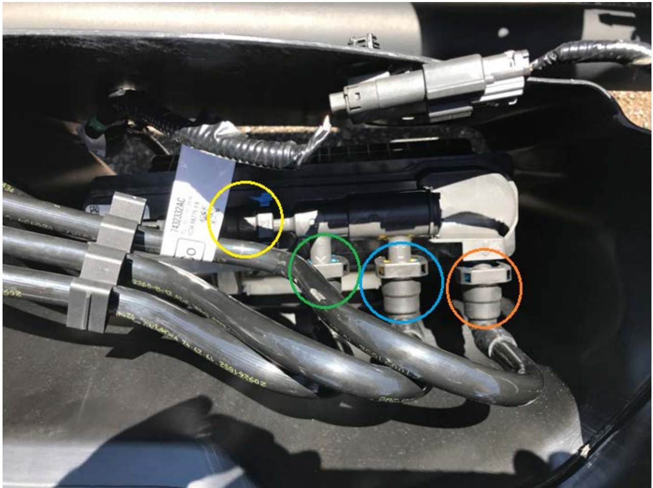
(Fig. 14) Water separator couplings showing color coding.
