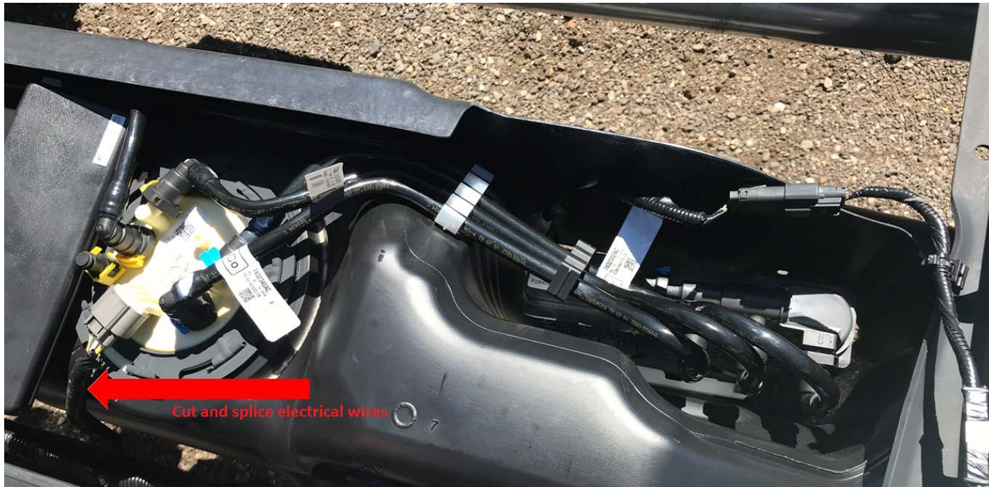
(Fig. 10) Using the wire kit supplied, cut and splice the sending unit electrical cable where shown by the arrow above so it will reach the rear, after-axle tank.
