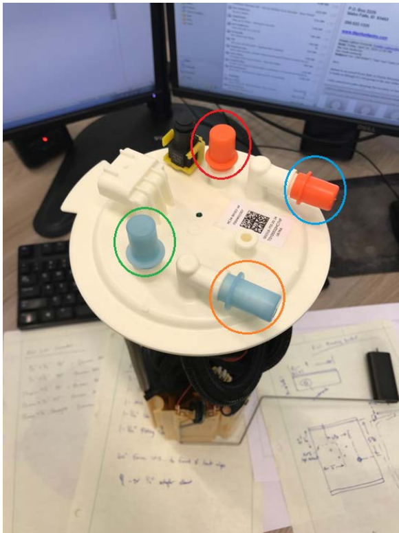
(Fig. 5) PFS-1147 Sending Unit showing the protruding tab, seen on the left and the color coding of the hose connections.
