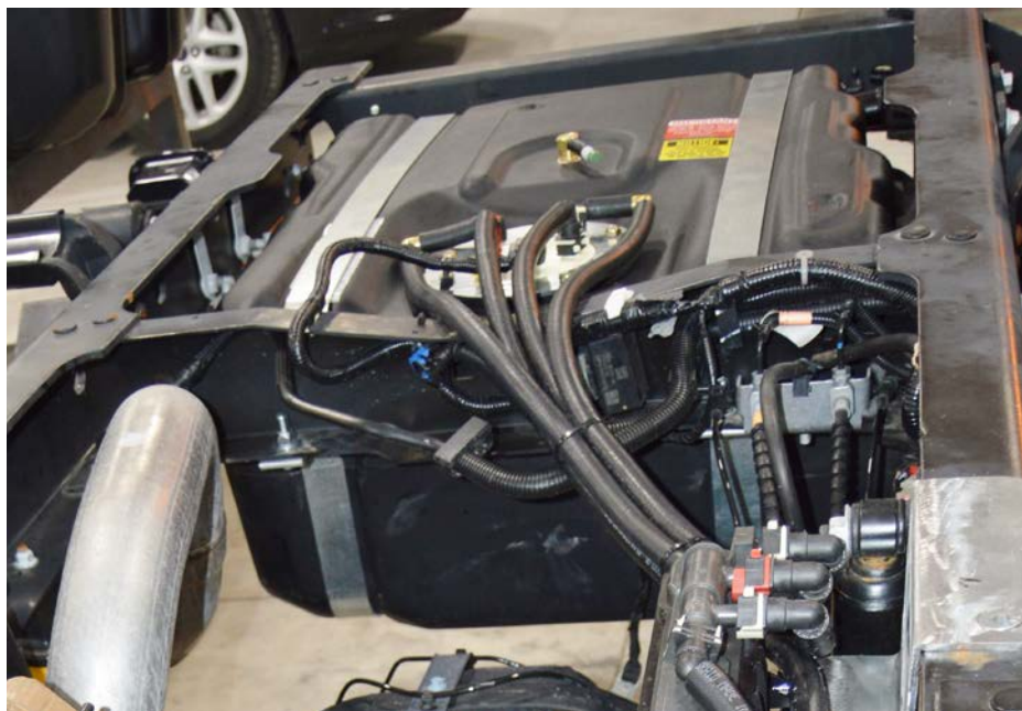
(Fig. 13) Front of TITAN tank, showing how tank straps are attached to the frame.
