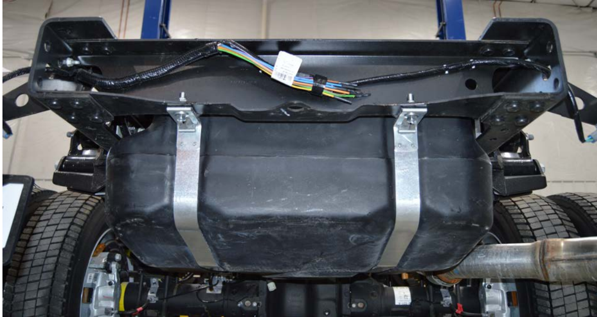
(Fig. 12) Rear of vehicle, showing how tank straps are attached to the frame.
