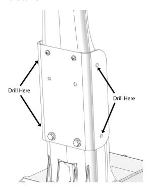
11. Secure the sides of the extension bracket to the stock tire carrier using ¼" bolts, flat washers and lock nuts.
