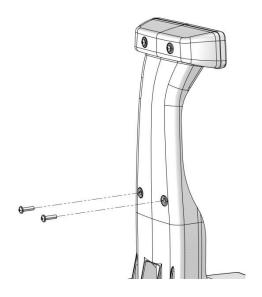
4. Secure the extension bracket on the stock tire carrier as shown in the picture below. Fasten the two factory screws removed in the previous step through the middle holes of the extension bracket into their original holes. Ensure that the middle holes in the extension bracket are offset away from the brake light as shown below.
