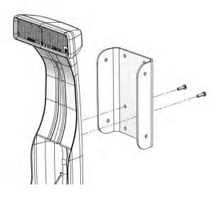
5. Using the holes in the extension bracket as guides, drill two ¼" holes in the tire carrier. Use the holes directly below the installed screws.
