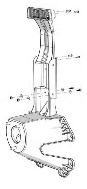
10. Using the holes in the sides of the extension bracket as guides, drill four ¼" holes in the stock tire carrier.
