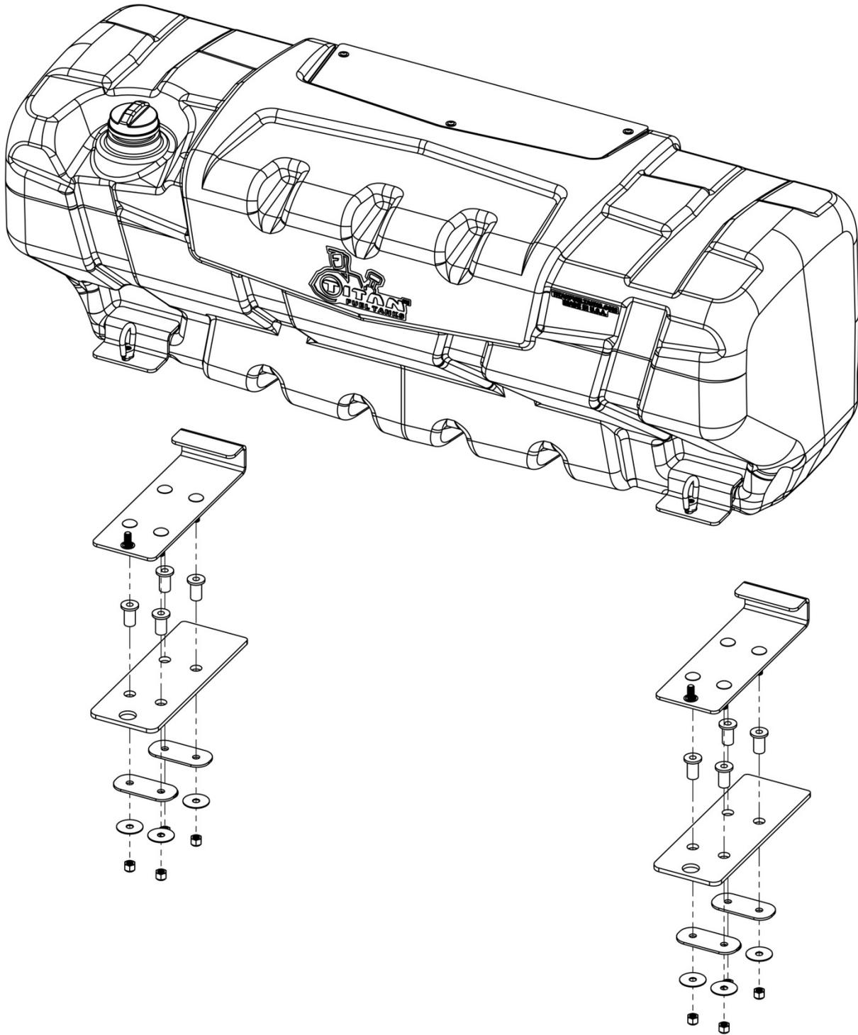
**This is an exploded view showing proper installation of the Aluminum Body Insulator Kit under the tank mounting brackets on top of; and Polymer Double Washers underneath the truck bed. Be sure to see *Travel Trekker 40™* Installation Instructions.**
