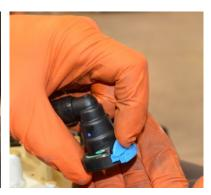
**Method for Disconnecting Ford Sending Unit Fuel Line Couplings:** The couplings on the sending unit are of the quick connect type shown in left photo above. To disconnect, a) Slide the tab that has teeth on its edge outwards as shown in the center photo. b) Next, press the rounded button, as shown in the right photo, and pull the coupling apart.
