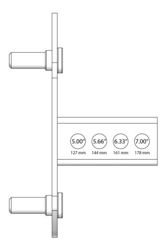
10. Slide the tire mounting bracket into the tank mounting bracket and secure with a 7/16" bolt, washers and locknut. Install the bolt through the hole in the tire mounting bracket determined in the previous step. Torque to 40 lb. ft. (54 N-m).
