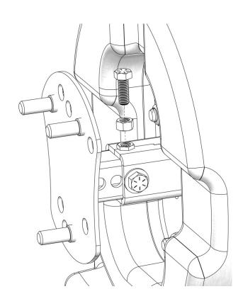
12. Install the spare tire onto the tire mounting bracket using the original lug nuts. Torque to 65 lb. ft. (88 N-m).
