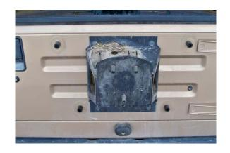
5. Attach the large ring terminal of the grounding wire to a mounting bolt. Be sure the bolt is connected to a metallic part of the vehicle's body or frame.
