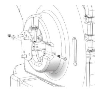
11. Thread the 3/8" X 1" bolt and hex nut into the weld nut on the tubing of the tank mounting bracket. Tighten the bolt and jam nut to 20 lb. ft. (27 N-m).
