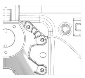
6. Attach the tank body to the tire carrier by securing the tank mounting bracket to the tire carrier wheel studs. Refer to the Mounting Templates on pages 10 and 11 of these instructions to determine which set of holes to use for your application. Secure with flat washers and lock nuts. Torque to 55 lb. ft. (75 N-m). Full tank weighs approximately 100 lbs (45 kg). Be sure mounting point is sufficient for weight.
