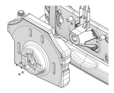
7. Press the provided wheel studs into the tire mounting bracket. Refer to the Bolt Pattern Templates on pages 12 and 13 of these instructions to determine which three holes to use for your vehicle.
